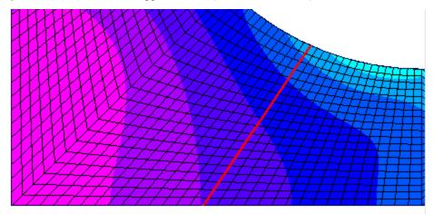
Output Set: Case 1 Time 1. Elemental Contour: Axisym Von Mises Stress
